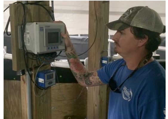
FOA Employee Using the 5500D Optical Dissolved Oxygen Instrument from YSI. Image credit: FOA.
